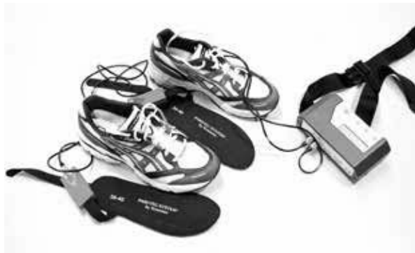
Figure 16.5 Pressure-measuring insoles are useful tools for measuring pressure on the plantar surface of the feet during gait.
