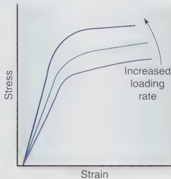
**FIGURE 11-2** Three stress–strain curves for cortical bone tissues tested in tension at three different loading rates. As the testing rate increases, the slope (the elastic modulus) of the initial straight line portion increases. (Adapted from Burstein AH, Wright TM. *Fundamentals of Orthopaedic Biomechanics*. Baltimore, MD: Williams & Wilkins, 1994:120.)
