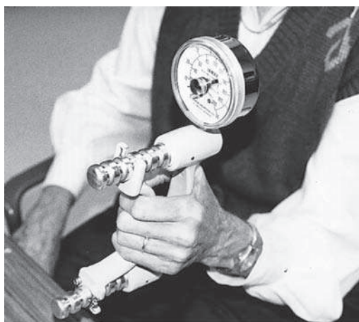
FIGURE 19.9 A Jamar dynamometer yields an objective measure of grip strength.
