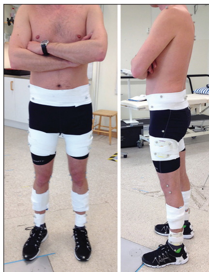
FIGURE 1. Lower extremity marker set used for analysis of the single-leg drop countermovement jump.
