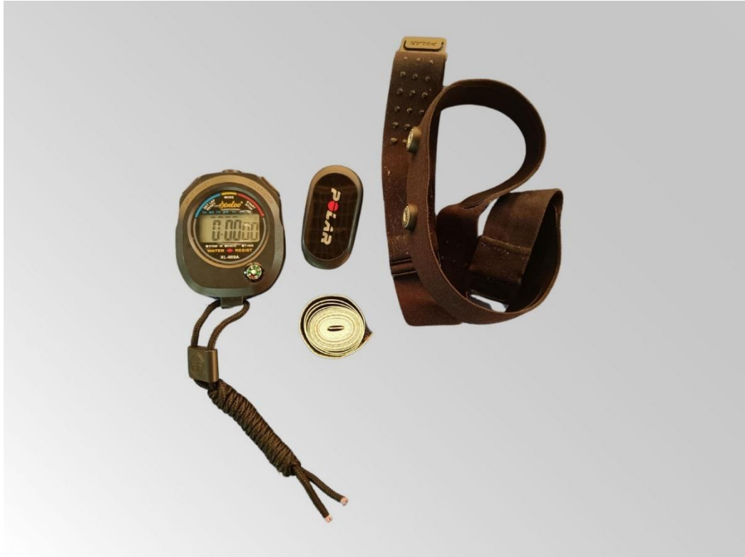
Fig3. Stopwatch, polar heart rate monitor along with the chest strap and measuring tape.
